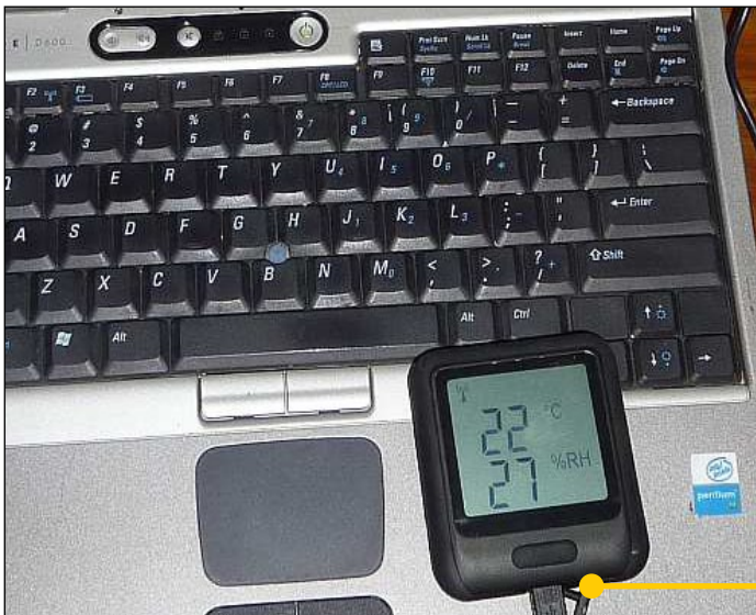
Figure 1 A networked temperature and humidity logger transmits data to a computer on the network. The difference in temperature between the logger and the computer occurred because the logger doesn't transmit in real time.
